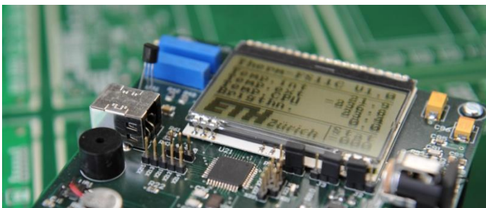
Digital thermometer board designed by students on the basis of a commercial microcontroller during the course "Applied Electrical Circuit and PCB Design".
